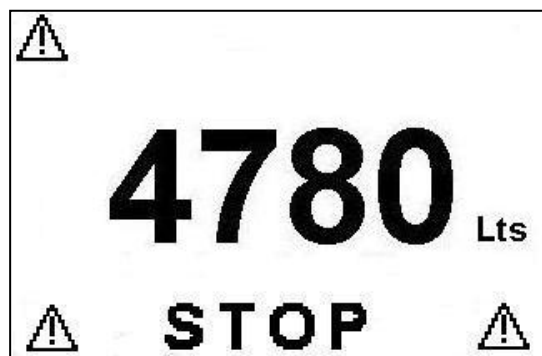
Figure 5 LCD – Overfill Alarm
