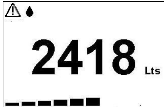
Figure 6 LCD – Bund Alarm
